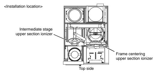
Note: The ionizer [optional accessory] is installed in only one of the locations.
