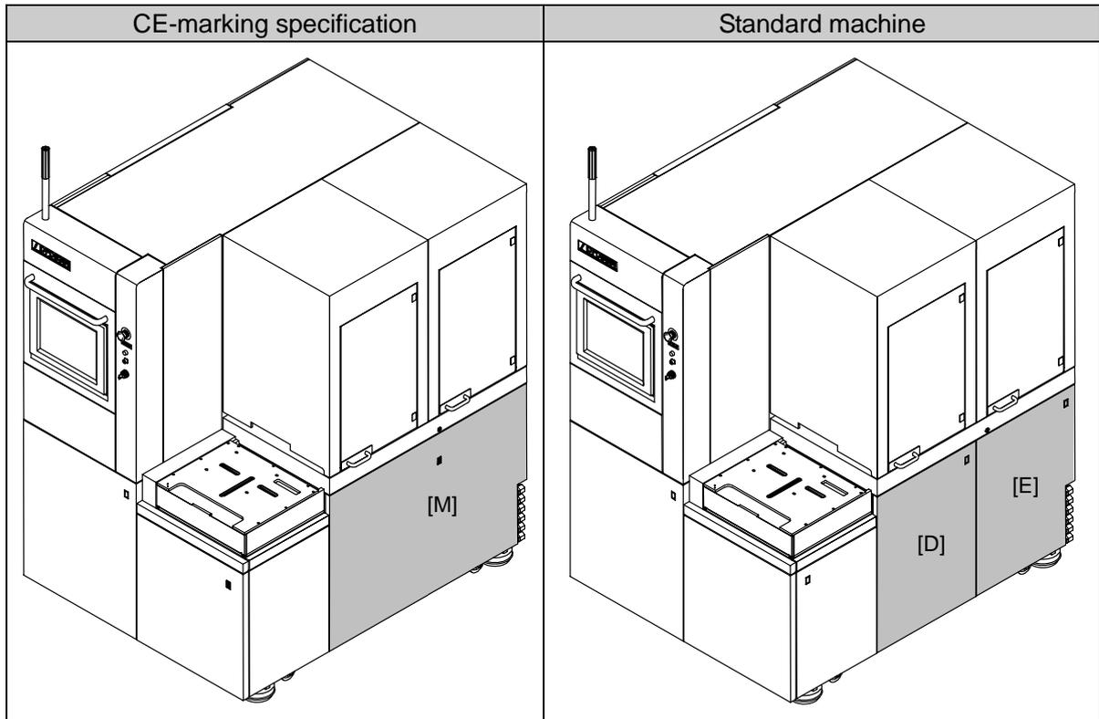
Interlock devices of the machine outer cover (The machine outer cover (partition (left), [P], [B], [M] and [R] cover) labeled with **COVER INTERLOCK** is equipped with interlock devices.)
